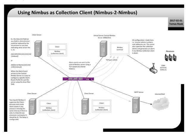
The above example shows four SCADA servers. In this case all SCADA are Citect servers but may be any kind of SCADA system Nimbus can import.
