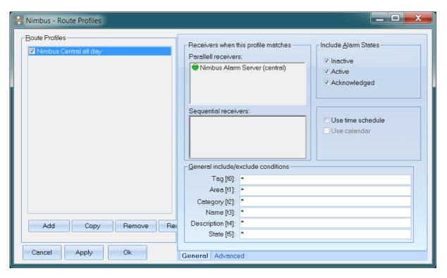
Create an *Alarm Route Profile*. The profile should normally send all alarm events to the previously created receiver. Select also *Acknowledged*. If needed some filtering may also be made here (ex only high prio alarms).
