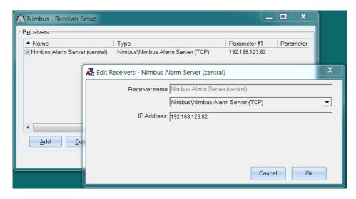
Create a *Receiver*, use the receiver type *Nimbus Alarm Server (TCP)*. There are multiple receiver types with similar names, ensure you select the correct one.
